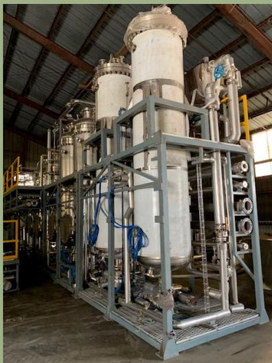
Acid Esterification of high FFA feedstock is one of the pre-processes that uses solid base BD-19 resin in a guard bed followed by multiple BD-20 resin beds. Resin beds can be recycled and reused.
